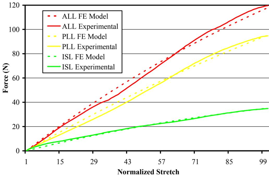
Figure 5: Ligament finite element models compared to the quasi-static experimental data for the ALL, PLL and ISL
