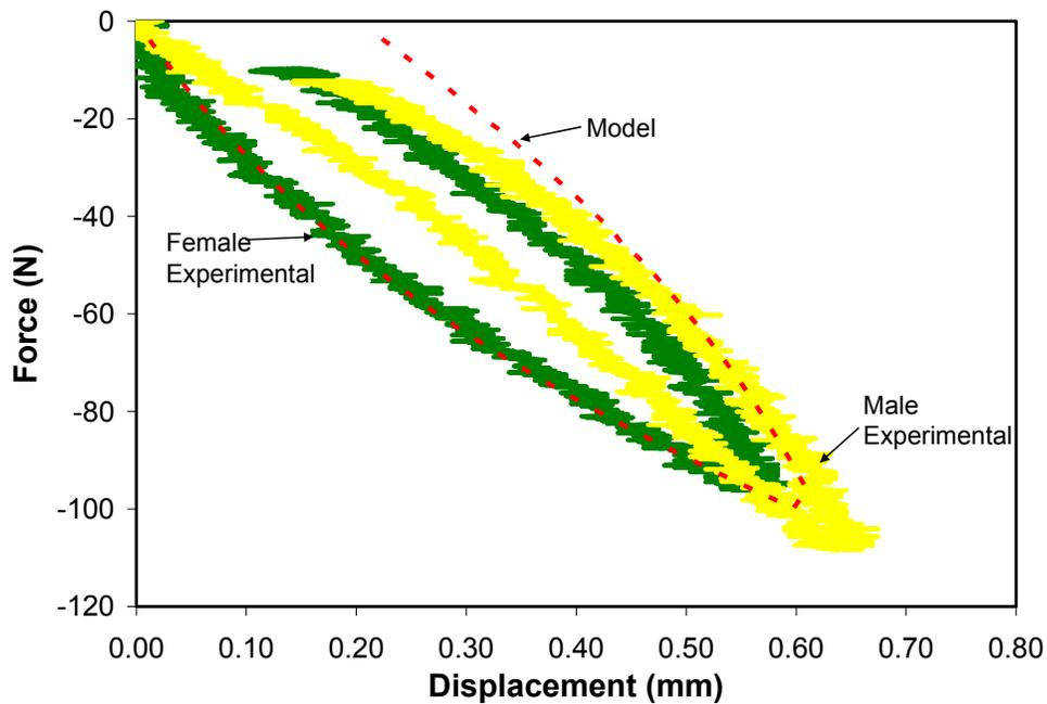
Figure 12: Disc finite element model compared to the experimental data for the disc in tension between two vertebral bodies
