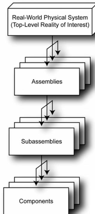
**Figure 1: Validation hierarchy illustrating the decomposition of a full system model into submodels (components, subassemblies, and assemblies)**
