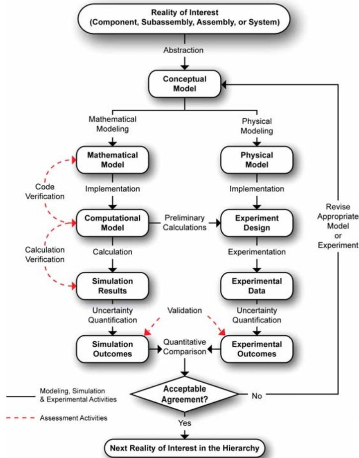
Figure 2: Detailed model development, verification and validation process
