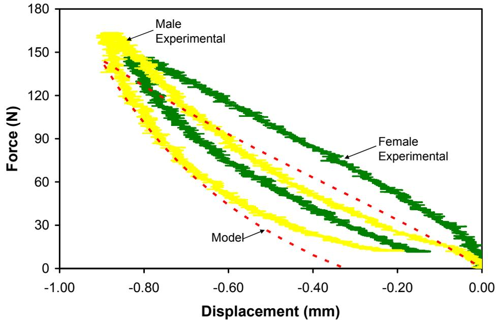
Figure 11: Disc finite element model compared to the experimental data for the disc in compression between two vertebral bodies
