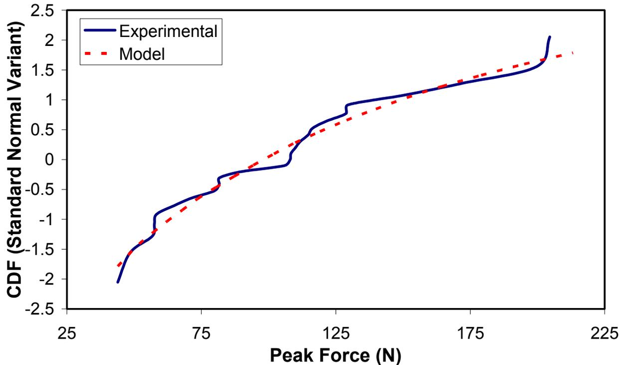
Figure 9: The experimental and model cumulative distribution functions of the maximum force during the relaxation test and simulation of the PLL
