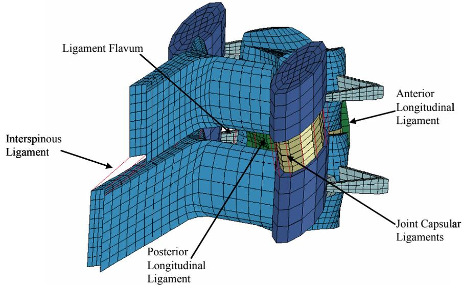
Figure 4: Motion segment model with the associated ligaments.
