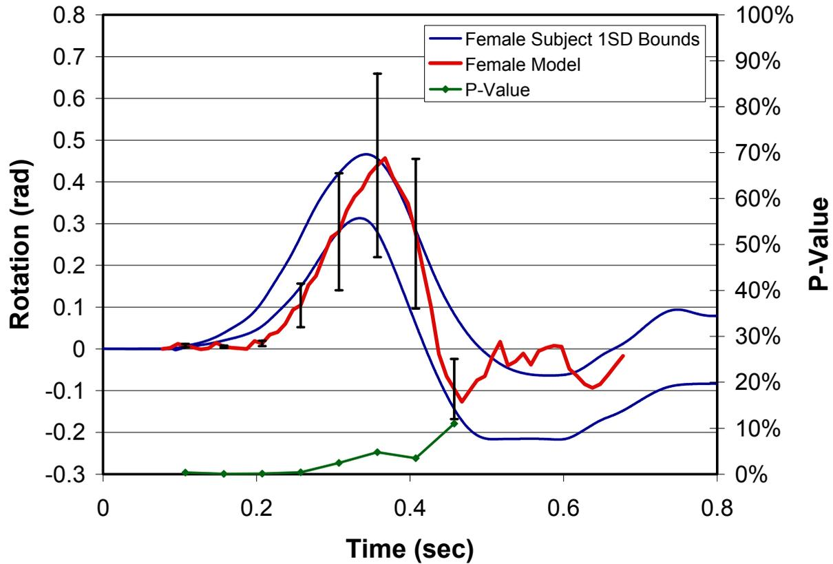
Figure 23: +5Gz ejection simulation head rotation for the full cervical spine probabilistic FE model. The one standard deviation corridors are shown for the experimental results as well as the probabilistic model response
