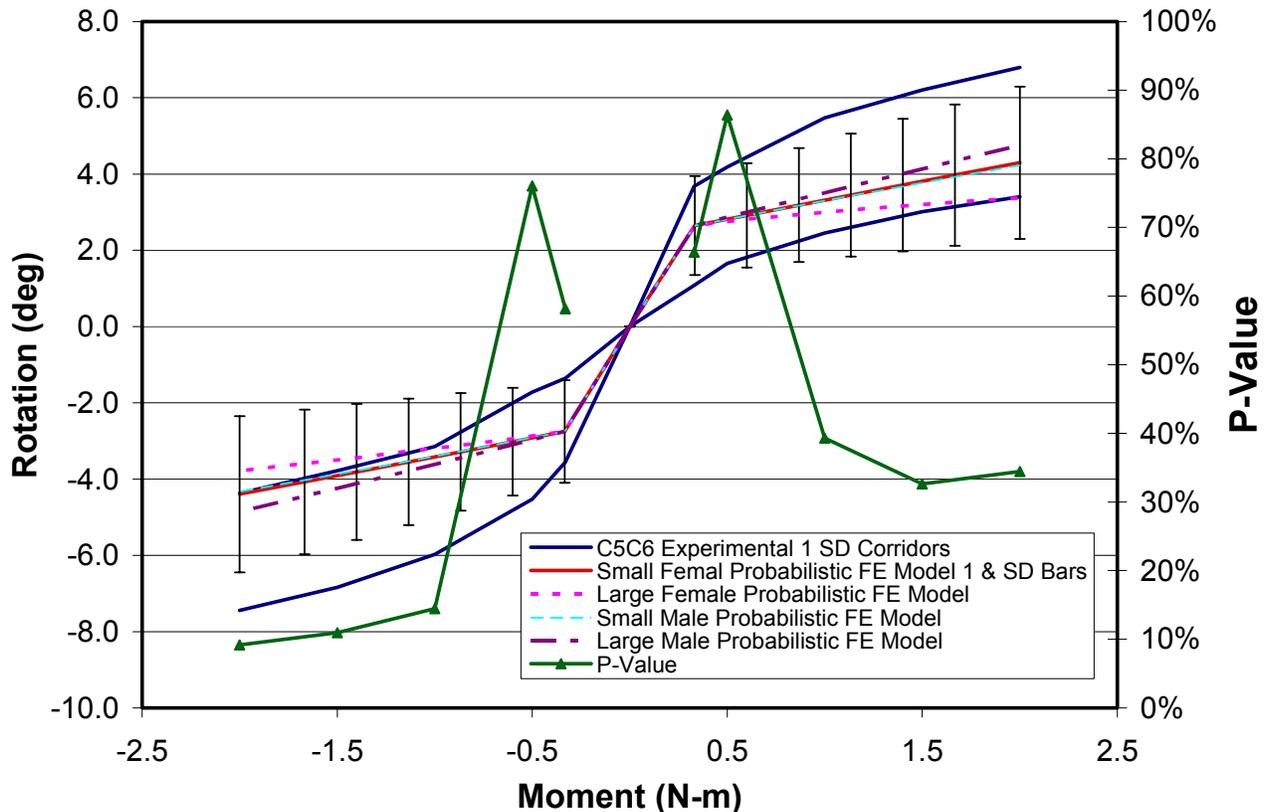
**Figure 16: Probabilistic response of a C5-C6 motion segment in lateral bending. Four models are shown representing large and small males and females. The one standard deviation corridors are shown for the experimental results as well as for the small female probabilistic FE model**
