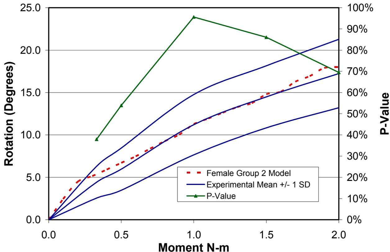
Figure 18: C3 extension rotation with respect to T1 mean value model response with one standard deviation corridors and mean experimental results
