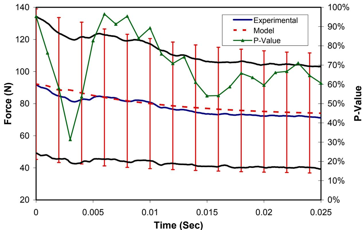
Figure 6: The experimental mean and one standard deviation corridors for the relaxation response of the ALL is shown with the mean and one standard deviation corridors for the probabilistic model response of the ALL
