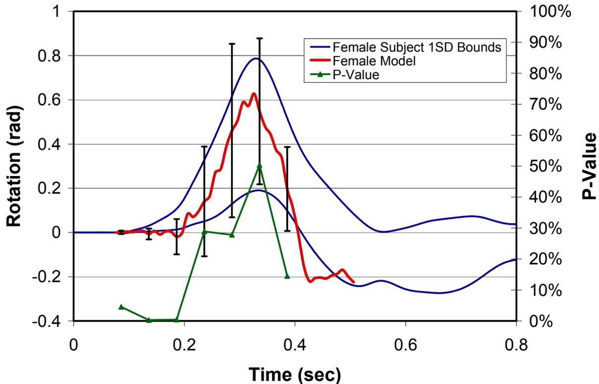
Figure 24: +7Gz ejection simulation head rotation for the full cervical spine probabilistic FE model. The one standard deviation corridors are shown for the experimental results as well as the probabilistic model response
