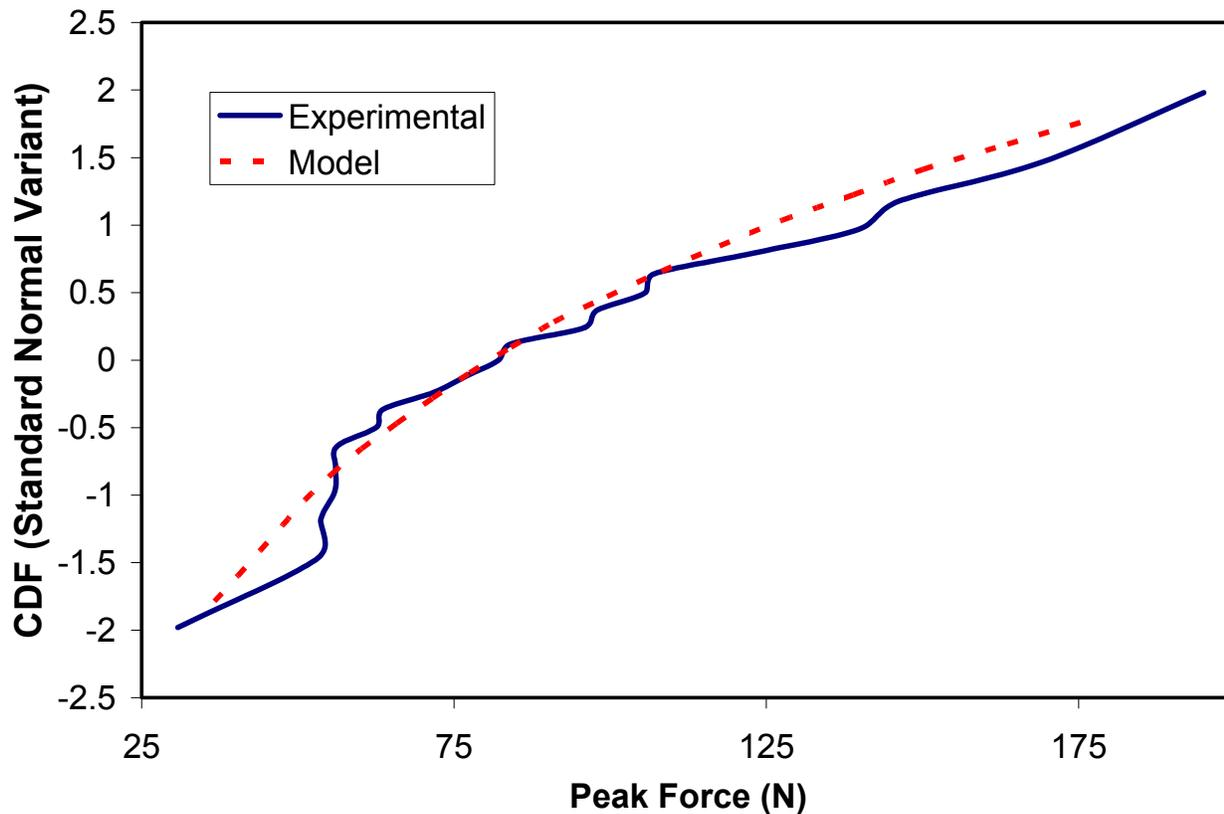
Figure 7: The experimental and model cumulative distribution functions of the maximum force during the relaxation test and simulation of the ALL
