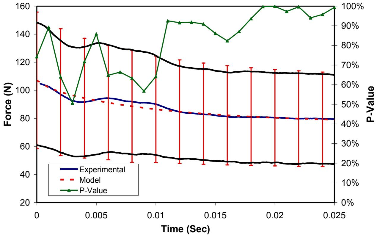
Figure 8: The experimental mean and one standard deviation corridors for the relaxation response of the PLL is shown with the mean and one standard deviation corridors for the probabilistic model response of the PLL
