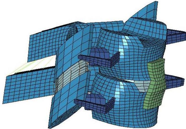
**Figure 13: Small female C5-C6 motion segment finite element model**
