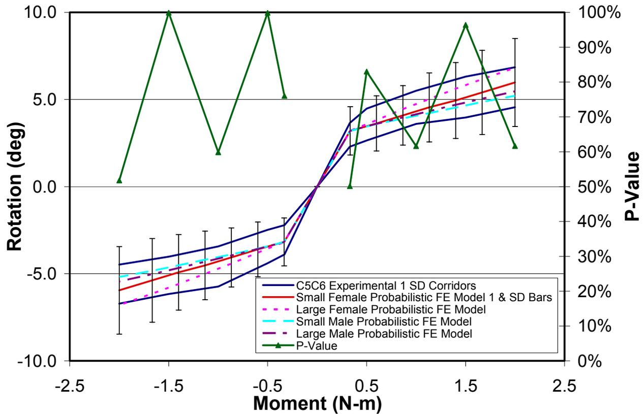
Figure 15: Probabilistic response of a C5-C6 motion segment in axial rotation. Four models are shown representing large and small males and females. The one standard deviation corridors are shown for the experimental results as well as for the small female probabilistic FE model
